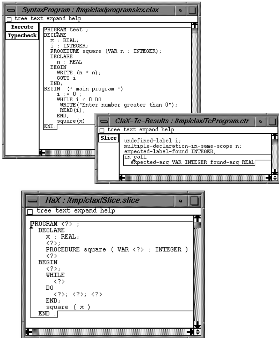
Figure 1: The CLaX environment. The top window is a program editor with two buttons attached to it for invoking a type checker and an interpreter, respectively. The middle window shows a list of four type errors reported by the type checker, in which the error message “in-call expected-arg VAR INTEGER found-arg REAL” is selected, indicating a mismatch between formal and actual parameter types in a procedure call. The bottom window shows the slice computed for this error message, containing all program components that contributed to the selected type error. The ‘<?’ symbols in the slice denote placeholders for program constructs not contributing to the error message.
