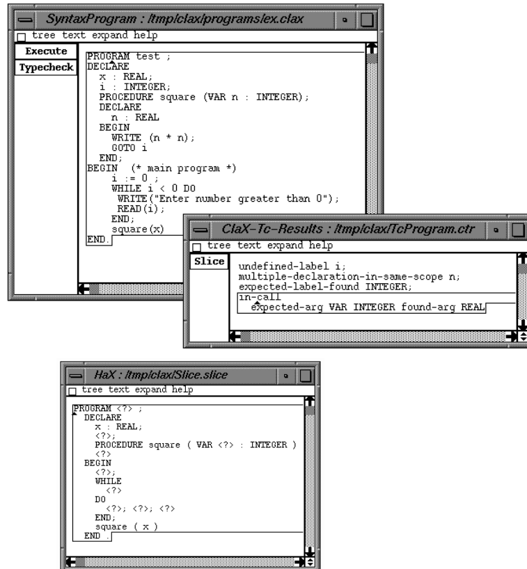
Figure 22: The ClaX environment. The top window is a program editor with two buttons attached to it for invoking a type checker and an interpreter, respectively. The middle window shows a list of four type errors reported by the type checker, in which the error message “in-call expected-arg VAR INTEGER found-arg REAL” is selected, indicating a mismatch between formal and actual parameter types in a procedure call. The bottom window shows the slice computed for this error message, containing all program components that contributed to the selected type error. The ‘<?>’ symbols in the slice denote placeholders for program constructs not contributing to the error message.
